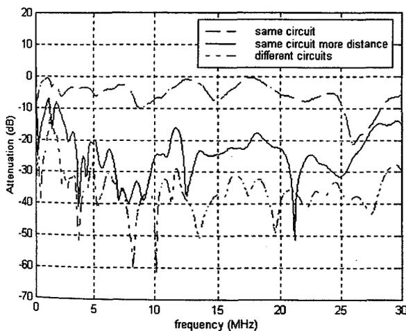
Figure 4: Amplitude response for three different channels measured in an apartment. Transmitter and receiver were located in different electrical circuits and positions.
