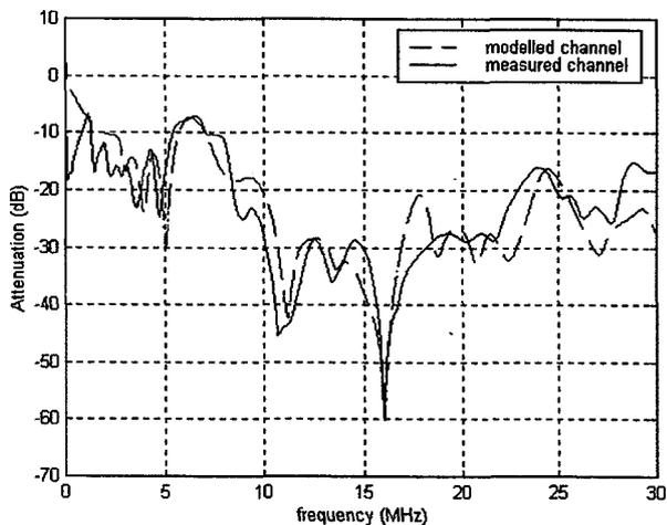
Figure 2: Example of channel amplitude responses obtained from the model and measurements.
