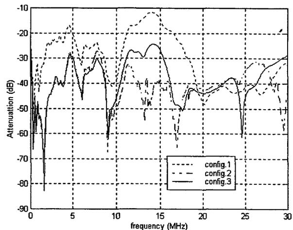
Figure 5: Amplitude response for a power line channel measured in the laboratory with different configurations of load.
