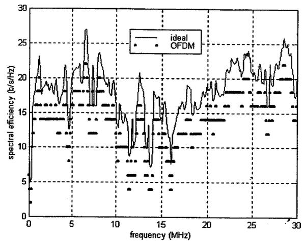
Figure 11: Respective channel capacity estimation.
