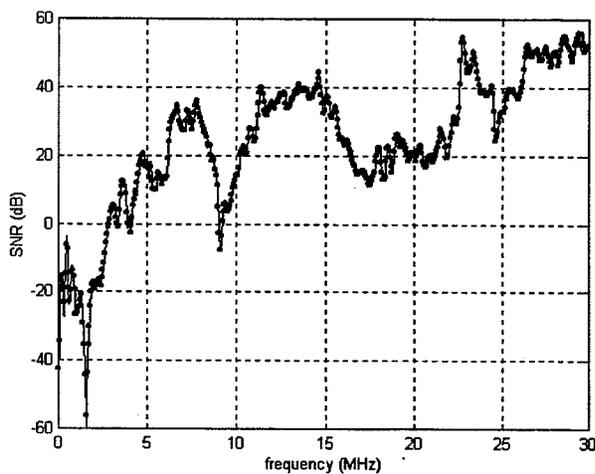
Figure 8: Channel signal to noise ratio for a laboratory measurement.
