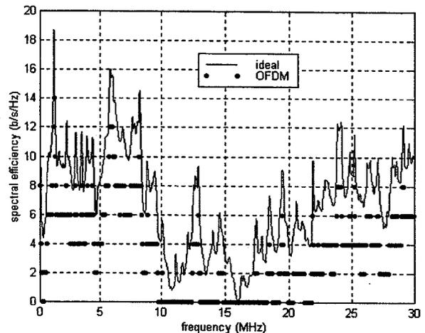
Figure 13: Respective channel capacity estimation.
