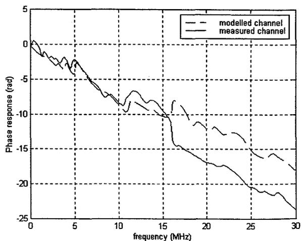
Figure 3: Example of channel phase responses obtained from the model and measurements.
