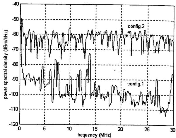
Figure 7: Noise measured in an apartment in the same situation, but in config.2 additional electrical appliances were turn on.
